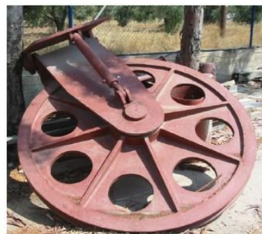
Fig. 1.17. Sheave suitable for electro-optical cable, 1.8 m diameter.
