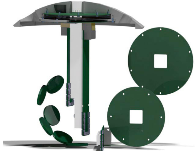
Figure 3-9: Layout of the electronic boards.
