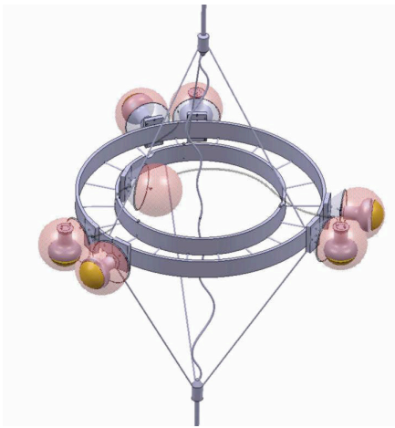
Figure 3-34: Triangle detection unit: detail of optical module and electronics sphere interconnections.
