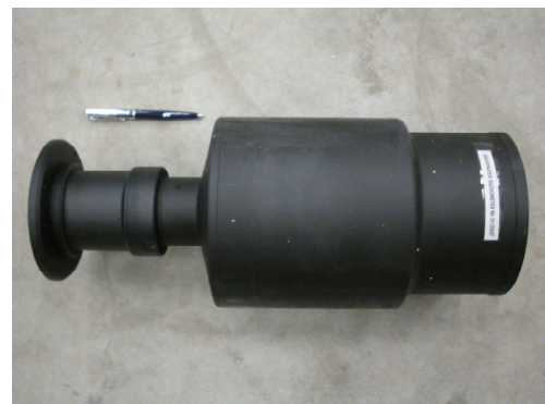
Figure 6-14: Probe for ^{40}\text{K} monitoring
