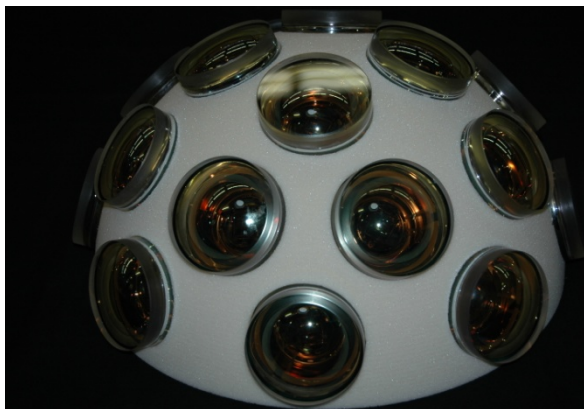
Figure 7-4: 20 3" photomultipliers in their Styrofoam support
