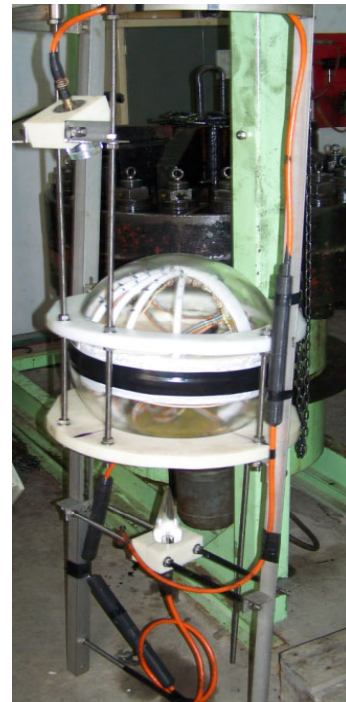
Figure 6-13: LIMS glass housing and mechanics
