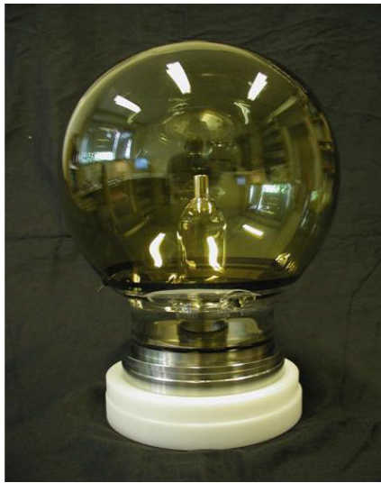
Figure 7-8: Spherical geometry X-HPD (8" prototype): (CERN-Photonis collaboration).
